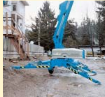
Optional Hydraulic Outriggers with Automatic Leveling System
